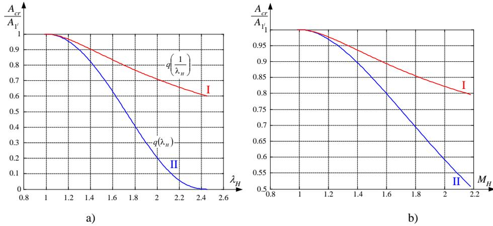
FIG. 4. Laval-type air intake starting limits
