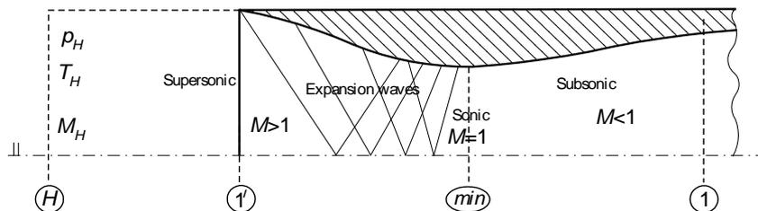
FIG. 1 Supersonic inlet with internal compression of inverted Laval type
